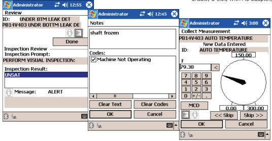
SKF MARLIN S-Pro IS CMDM 5360 ATEX Zone 1 certified Machine Reliability Inspection device
