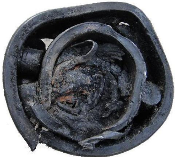
Premature bearing failure due to contamination problem
