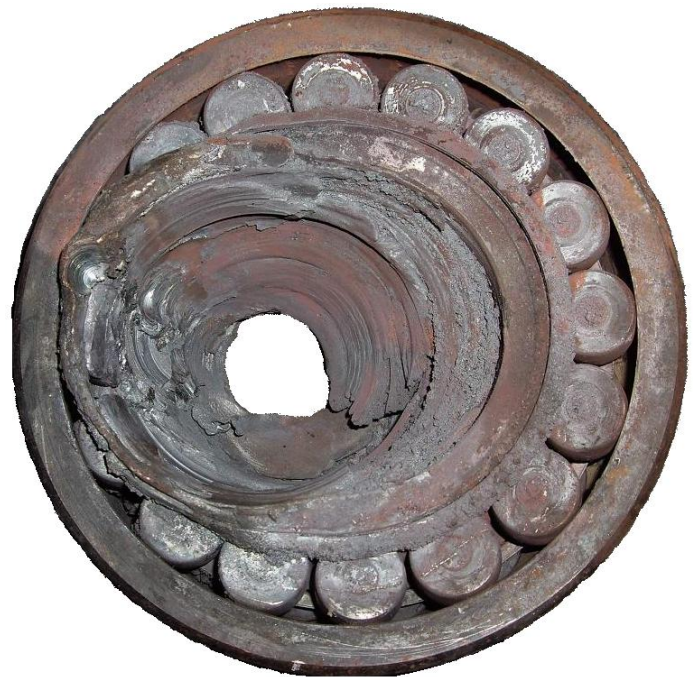
Premature bearing failure due to lubrication problem
